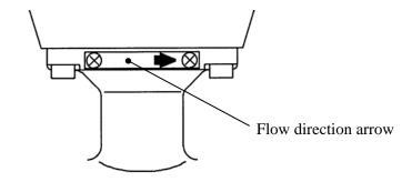
Figure 4.9 Flow direction arrow on the detector
